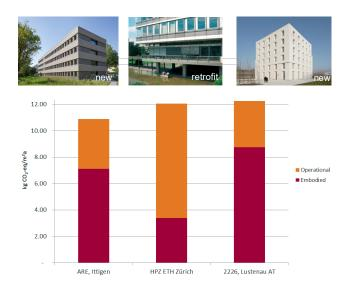
Embodied and operational greenhouse gas emissions (kg  $CO_2$ -eq per  $m^2$  and year) of three office buildings in Switzerland and Austria (two new and one retrofit building); lifetime: 60 years Source: Tschümperlin et al. 2016
