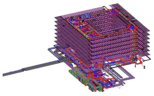
Figure 33: The BIM model of the HVAC systems of the case study building
