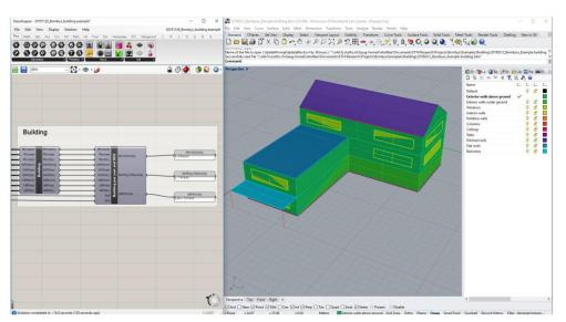
Figure 52: Bombyx plug-in in GH (left) and geometry with pre-defined layers (right).
