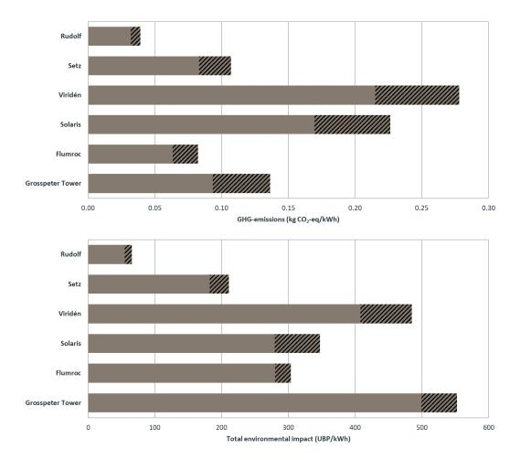
**Figure 5:** Gross greenhouse gas emissions (in kg CO<sub>2</sub>-eq, top) and gross environmental impacts (in eco-points, bottom, see also case study 1.3D3-01) per kWh electricity produced by the active glass façades of six BIPV buildings. The shaded area can be attributed to the building (impacts of front glass and supporting structure) and not the electricity production.
