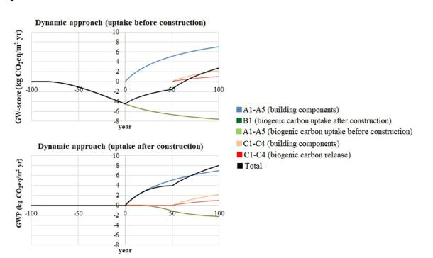
Figure 10: Global warming (GW) scores of the analyzed building as a function of the reference service life (year 0 is the construction of the building).
