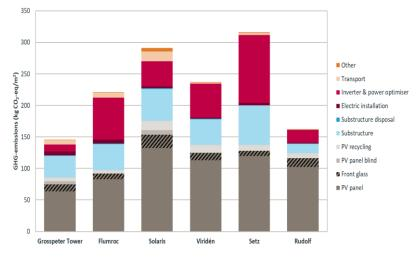
Figure 4: Greenhouse gas emissions per m<sup>2</sup> active glass façade of the six selected buildings divided into the impacts associated to PV panels, blind PV panels, substructure, disposals of PV panels and substructures, balance of system (BOS), transport and other (edge seals, joints). Note: Office buildings: Grosspeter Tower, Flumroc. Residential buildings: Solaris, Viridén, Setz, Rudolf.
