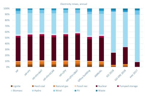
**Figure 3:** Technology shares of the annual Swiss electricity mixes for the different load profiles of the residential building Rautistrasse, the load profile of the ARE office building, the annual Swiss electricity mix (national load profile) and the Swiss consumer electricity mix 2018 according to guarantees of origin.
