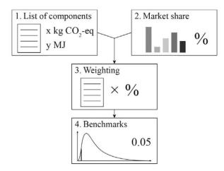
Figure 16: Simplified input on building level using the four categories as drop-down selections
