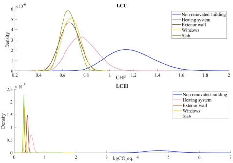
**Figure 23:** Measures applied following each iteration of the sensitivity analysis. The top graph shows results of uncertainty quantification for LCC in total CHF (Swiss Franc). The lower graph shows results of uncertainty quantification for LCEI (Life Cycle Environmental Impact) in total kg CO<sub>2</sub>eq.
