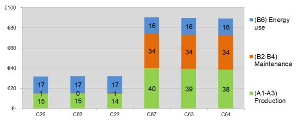
Figure 6: NPV of the total environmental cost of the three flat roof alternatives with best and worst performance (6 alternatives) within the total of the 114 alternatives assessed.
