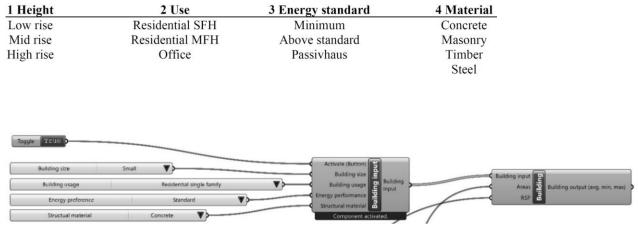
Figure 25: Simplified input on building level using the four categories as drop-down selections. SFH = single-family house; MFH = multi-family house
