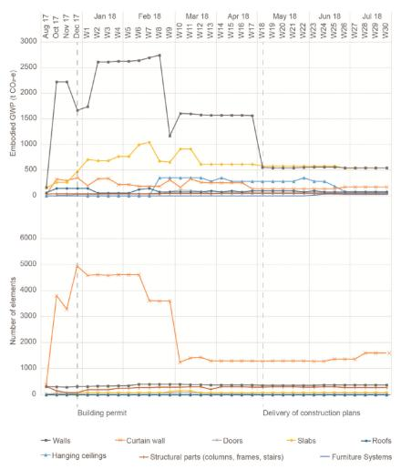
Figure 47: Evolution of results for embodied GWP in t CO<sub>2</sub>-e for individual building elements and number of elements throughout the design process.
