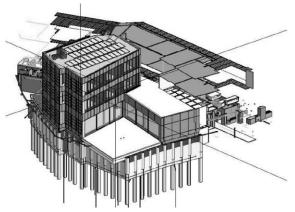
Figure 46: Example BIM model for the case study – the first office building in Switzerland built without printed plans
