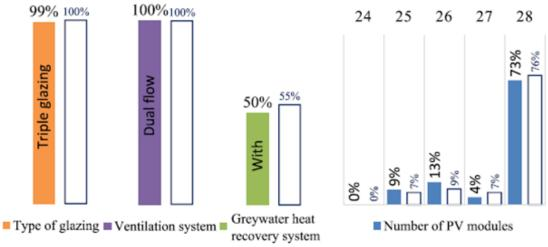
Figure 57: Examples of statistical analysis on optimal solutions. Note: The white bars correspond to a calculation of all possible parameters combinations (over 4 millions) and the coloured bars to the results of the genetic algorithm (8,000 calculations). Both Pareto fronts provide similar trends.
